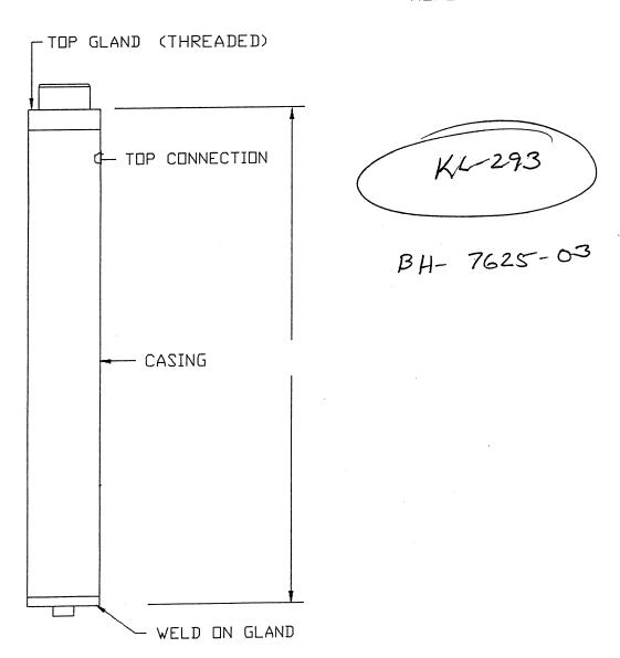
NDTE: This is the second generation of the 70/90 cylinder. It has the hydraulic line connection at the top and a threaded gland. It does not have a slot like the 1086088. This cylinder can be repacked with KL-284
