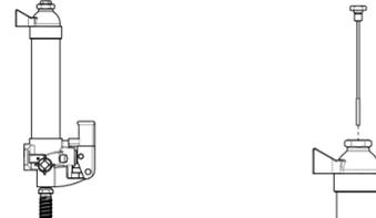
2. Turn the Pump Unit on its side so that old oil will drain from the oil fill hole.
