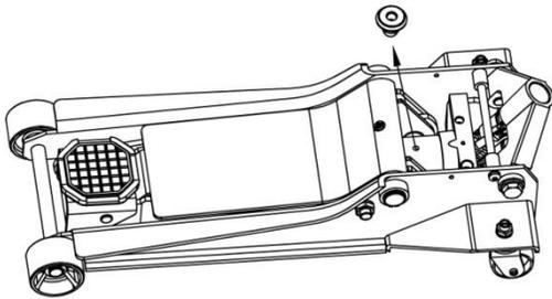
4. Fill the oil case until oil level is just beneath the lower rim of the oil fill hole.
