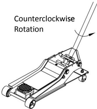
3. Rapidly pump the handle 6-8 times. Leave handle in down position to expose oil fill plug.
