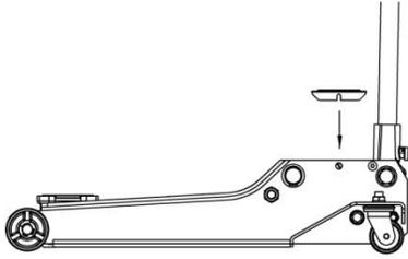
6. Turn release valve clockwise to the closed position.
