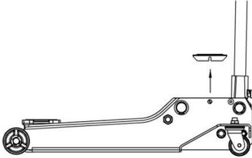
2. Turn release valve **counter-clockwise** on full turn to the open position.
