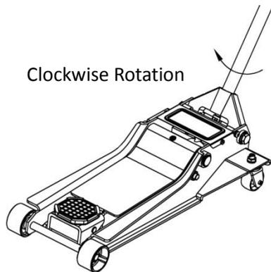
7. Before raising the vehicle double check and verify the saddle is centered and also has full contact with the lifting point.
