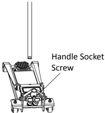
5. Line up the square whole located at the bottom of the handle over the square bolt inside the Handle Socket.
