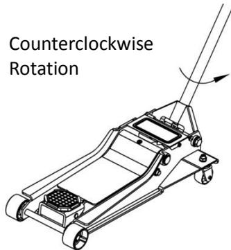
5. After removing jack from under the load, keep jack in the lowered position to reduce exposure to rust and contamination.
