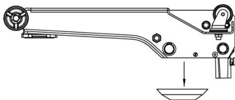
6. Position the jack on level ground and keep saddle in the lowered position. Fill the oil case until oil level is just beneath the lower rim. Keep dirt and other foreign materials clear when pouring.
