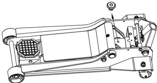
5. Turn the jack on its side to drain old oil from the oil fill hole.
