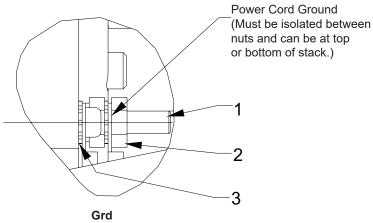
Note: Serrated lockwasher must be adjacent to pump body.
