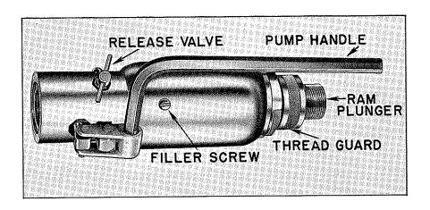
If you use HYDRA-RAM without attachments, be sure to use the serrated plunger saddle (BJ-10-13) as in Illustration A, the thread guard
