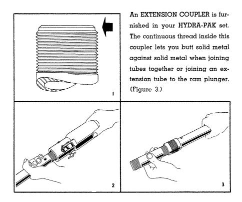
KWIXTENSION saves time in making a setup on the job. An exclusive feature in HYDRA-PAK, this extension attachment gives you 14 positions with quick extensions from 4" to  $11\frac{3}{4}$ " length. No need to change extensions on a body job or other work of less than six tons — a pull on the pad end extends the KWIXTENSION to any of the 14 positions. To retract, just lift the knurled knob and slide the extension back to its original length (Figure 4)
