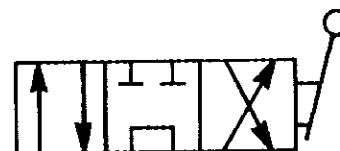
4 WAY VALVE TANDEM CENTER
