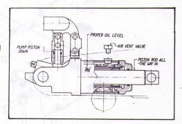
Adding Oil: With Saddle fully lowered & jack on level ground, Remove cover plate then remove Air Vent Valve. Oil level should be approx. 3/16" below valve hole. If low, add oil as needed. Replace cover plate.
