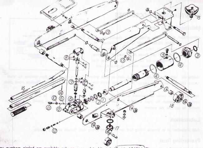
The key numbers circled are available only as a complete kit under Part # 124614. They cannot be ordered individually. The description and quantity of the components that make up this kit are shown below. The key numbers not circled identify the only components available as individual parts.
