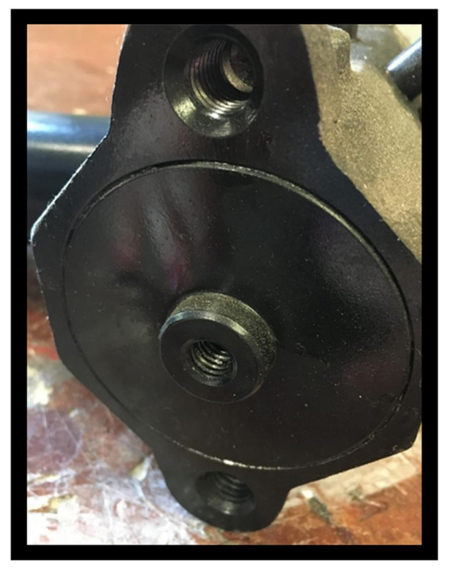
The holes in the end caps are threaded. The end caps are press fit into the reservoir. We find a bolt with matching threads and partially thread the bolt into the holes in the center of the end caps. Then, using a wrench on the bolt, jiggle loose the end cap. You can also knock the bolt with a mallet to loosen the end caps.
