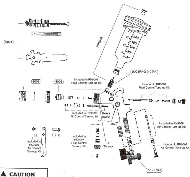
**DO NOT REMOVE Brass** Baffle Attached to Front of Body of Gun (See Parts Diagram). Special Technical Training and Tools are Required. Only Authorized Service Centers **Should Remove This** Part.
