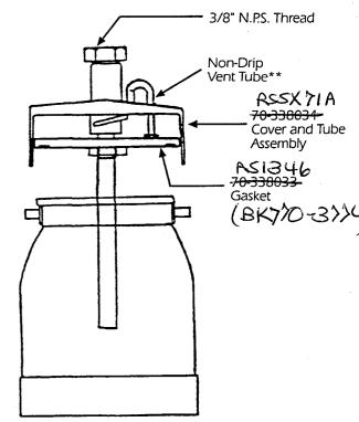
\*\* Note: If a replacement for the Non-Drip Vent Tube is needed, use a length of 5/32" I. D. nylon tubing
