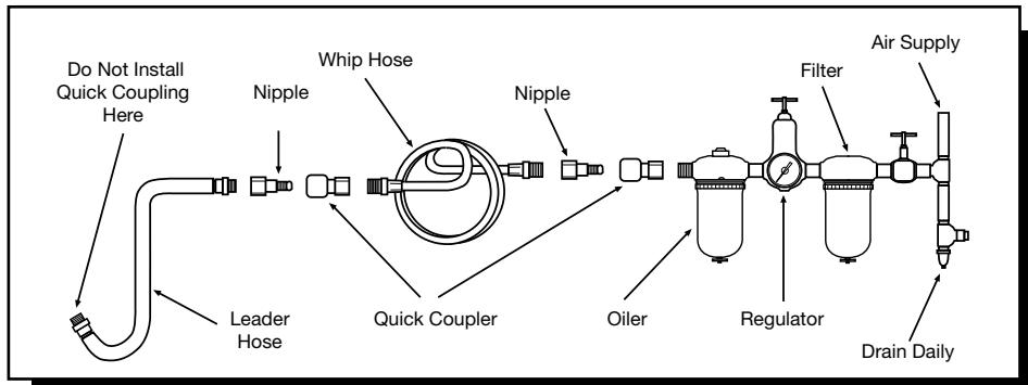
Tools operate on a wide range of air pressures. We recommend that air pressure measures 90 PSI at the tool with the trigger fully depressed and no load applied to the tool. Low pressure (less than 90 psig 6.2 bar) reduces the speed and performance of all air tools. High pressure (over 115 psig 8.0 bar) exceeds the rated capacity of the tool, which will shorten tool life and could cause injury.
