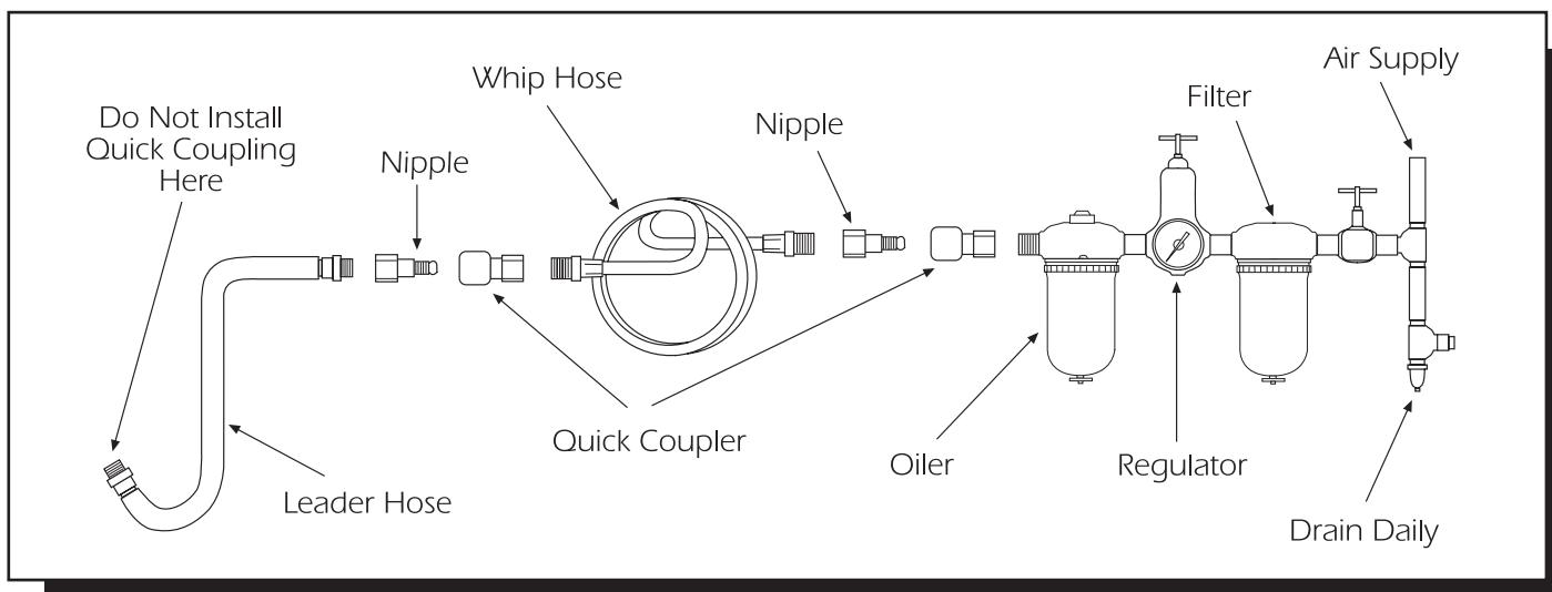
Tools of this class operate on a wide range of air pressures. It is recommended that air pressure of these tools measures 90 PSI at the tool while running free. Low pressure (under 90 psig; 6.2 bar) reduces the speed of all air tools. Low air pressure not only wastes time, but also costs money. Higher pressure (over 90 psig; 6.2 bar) raises performance beyond the rated capacity of the tool, which will shorten tool life because of faster wear and could cause injury. Always use clean, dry air.
