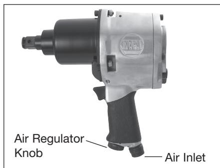
The air inlet used for connecting air supply, has standard 1/4" NPT American Thread. Line pressure should be increased to compensate for unusually long air hoses (over 25 feet). Minimum hose diameter should be 1/2" I.D. and fittings should have the same inside dimensions and be tightly secured.
