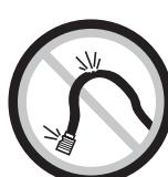
off the air supply, drain hose of air pressure and detach tool from air supply before installing, removing or adjusting any accessory on this tool, or before performing any maintenance on this tool. Failure to do so could result in injury. Whip hoses can cause serious injury. Always check for damaged, frayed or loose hoses and fittings, and replace immediately. Do not use quick detach couplings at tool. See instructions for correct set-up.
