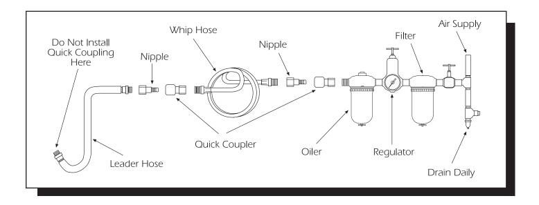
Tools of this class operate on a wide range of air pressures. It is recommended that air pressure of these tools measures 90 PSI at the tool while running free. Low pressure (under 90 psig; 6.2 bar) reduces the speed of all air tools. Low air pressure not only wastes time, but also costs money. Higher pressure (over 90 psig; 6.2 bar) raises performance beyond the
