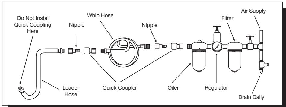
Tools operate on a wide range of air pressures. We recommend that air pressure measures 90 psig at the air inlet with the trigger fully depressed and no load applied to tool. Low pressure (less than 90 psig 6.2 bar) reduces the speed and performance of all air tools. High pressure (over 115 psig 8.0 bar) exceeds the rated capacity of the tool, which will shorten tool life and could cause injury.
