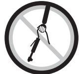
• Tool shaft may continue to rotate briefly after throttle is released. Avoid direct contact with accessories during and after use. Gloves will reduce the risk of cuts or burns.
