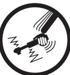
Air-powered tools can vibrate during use. Extended exposure to vibration, repetitive motions, or uncomfortable positions during use may be harmful to your hands and arms. Discontinue use of tool if discomfort, tingling, or pain occurs. Seek medical advice before resuming use.
