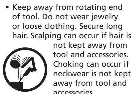
• Keep away from rotating end of tool. Do not wear jewelry or loose clothing. Secure long hair. Scalping can occur if hair is not kept away from tool and accessories. Choking can occur if neckwear is not kept away from tool and accessories.
