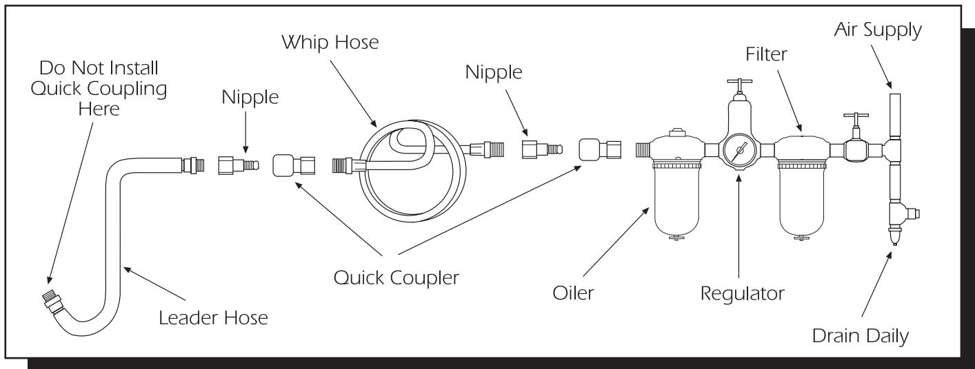
Tools of this class operate on a wide range of air pressures. We recommend that air pressure measures 90 PSI at the air inlet while in use. Low pressure (less than 90 psig/6.2 bar) reduces the speed and performance of all air tools. High pressure (over 115 psig/8.0 bar) exceeds the rated capacity of the tool, which will shorten tool life through faster wear and could cause injury.
