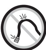
Whip hoses can cause serious injury. Always check for and replace any damaged, frayed, or loose hoses and fittings. Do not operate a damaged or worn tool. Do not use quick-detach couplings at tool. See instructions for correct setup.
