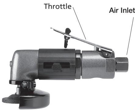
The air inlet used for connecting the air supply has standard 1/4" NPT American Thread. Line pressure should be increased to compensate for unusually long air hoses (over 25 feet). Minimum hose diameter should be 3/8" I.D. Fittings should have the same inside dimensions and should be tightly secured.
