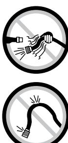
serious injury. Always check for and replace any damaged, frayed or loose hoses and fittings. Do not operate a damaged or worn tool. Do not use quick-detach couplings at tool. See instructions for correct set-up.
