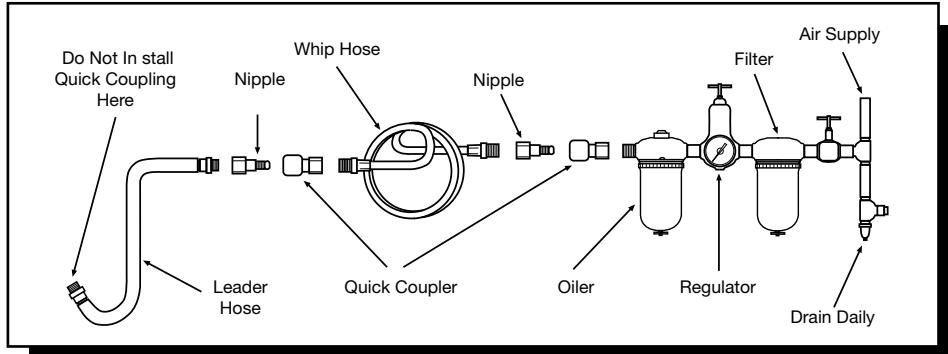
Tools of this class operate on a wide range of air pressures. We recommend that air pressure measures 90 PSI at the air inlet while in use. Low pressure (less than 90 psig 6.2 bar) reduces the speed and performance of all air tools. High pressure (over 115 psig 8.0 bar) exceeds the rated capacity of the tool, which will shorten tool life through faster wear and could cause injury.
