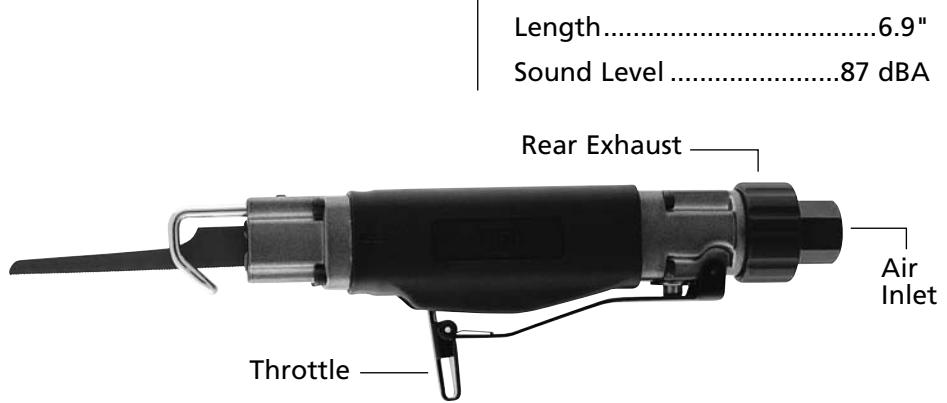
The air inlet used for connecting air supply, has standard 1/4" NPT American Thread. Line pressure should be increased to compensate for unusually long air hoses
