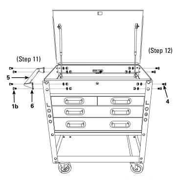
**Step 13:** Insert the remaining 8 stove bolts (Part #1a).
