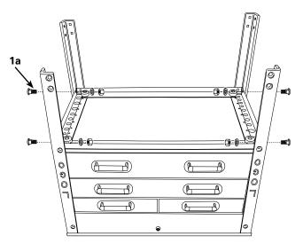
Step 6: Completely tighten the 8 bolts just inserted.
