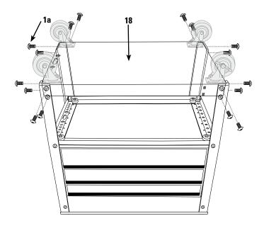
Step 8: Carefully lift cart onto its casters.
