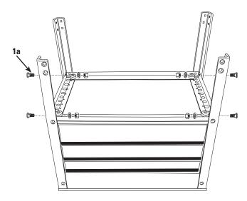
Step 7: Insert bottom shelf (Part # 18) between the four legs flat side facing up towards the ceiling. Insert sixteen stove bolts (Part #1a) and completely tighten.
