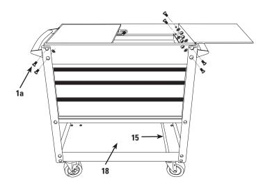
Step 13: Using 13mm socket completely tighten all fasteners!!
