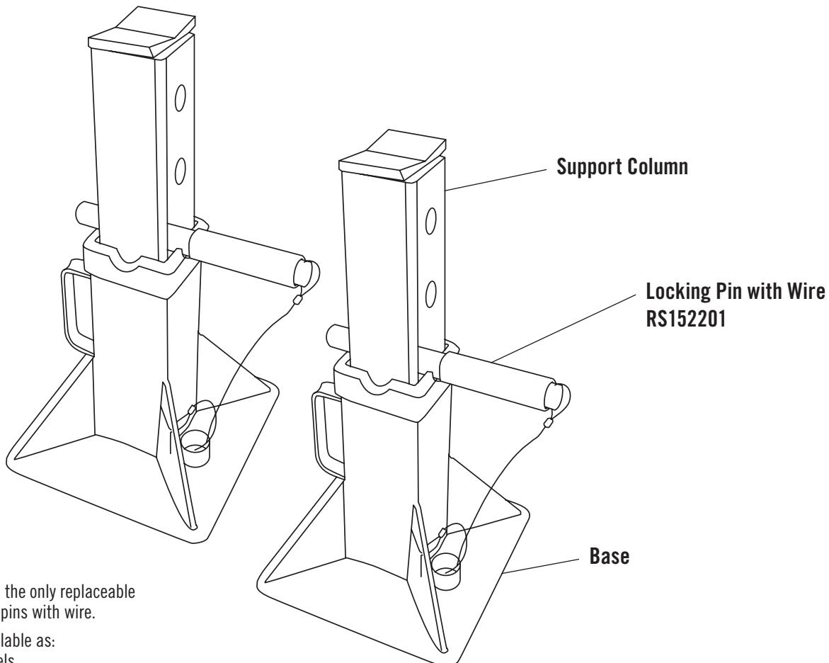
Due to safety precautions, the only replaceable part is RS152201, locking pins with wire.
