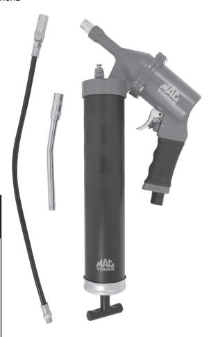
Continuous Shot Air Grease Gun is a fully pneumatic powered tool. The gun is designed for lubrication of grease points in automotive and truck applications. The gun has a single action pump that delivers grease each time the trigger is depressed and the plunger moves forward.
