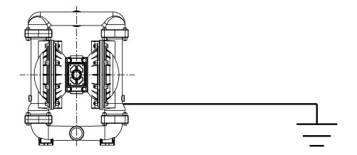
This 8 foot long (244 centimeters) Ground Strap (Item 32) is shipped with the eyelet end fastened to the pump hardware.
