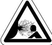
*Before maintenance or repair, shut off the compressed air line, bleed the pressure, and disconnect the air line from the pump. The discharge line may be pressurized and must be bled of its pressure.*
