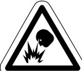
*Take action to prevent static sparking. Fire or explosion can result, especially when handling flammable liquids. The pump, piping, valves, containers or other miscellaneous equipment must be grounded. (See page 21)*
