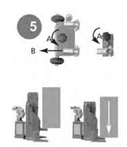
Lifting and lowering using an external pump:
