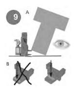
If you lift one side of a top-heavy object the load could top over (A). Watch the angle of the load carefully - if you see problems lower the load and use more than one toe jack and/or re-think the lifting plan.
