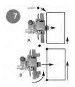
In cases where the swiveling legs have no space you should consider the following: Spread the legs to the outside (never to the back) and lift the load above the height of the legs
