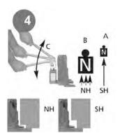
Fast stroke SH (only 25 ton) with 3-times the speed of the regular stroke NH.  $\,$
