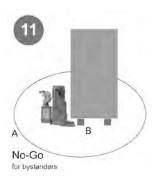
Always make sure that bystanders and children are away from the work area. Cordon off a NO-GO area with cones and tape, etc. The NO-GO area must be the area of the load plus a radius around the load of at least 1.5 times the highest dimension of the load. This is the operators' responsibility (A). Make sure the load is supported during the lifting and lowering process, and that the load
