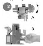
When using the Jack you should always: Put the swiveling legs to the front of the jack (A) Then locate the lifting toe in the correct position (B). To do this you have to lift up the toe assembly, pull it out and push it back into the desired position and lower the toe until it cannot go down any further.
