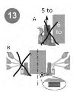
The jack will not lift loads above the rated capacity due to the built in safety valve (A). If you use more than one jack you should support the load gradually step by step (see diagram) to prevent an unbalanced load with different loads on each jack. Failure to do so could cause an overload on one jack and the load might tip (B).
