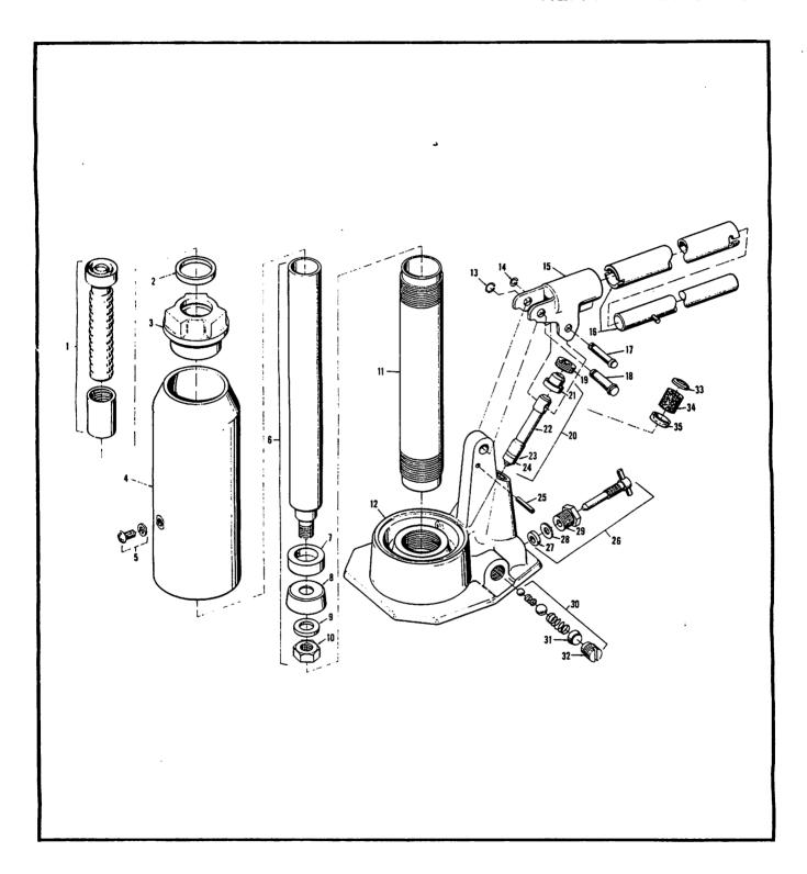
Item numbers shown above are only for your convenience in locating the part on the parts list. When ordering, always specify the PART NUMBER — not the item number — and give complete name of part and model number of jack. If the length of the part is shown on the parts list, verify it with the old part. If different, state exact length and diameter of old part.
