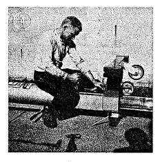
Pull base assembly "out" to obtain access to the two stop block bolts.
