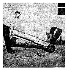
Standing behind the lift, grasp the top of the cylinder and tip down and toward you, pivoting on the rubber wheels, and locating so that the safety stop bracket will be supported on the saddle post previously placed on the floor. (See Fig. 3).
