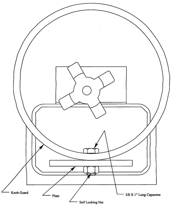
Install the Knob Guard on top of the plate welded to the back of the power unit reservoir. If there is not a hole in the plate you will need to drill a 7/16" diameter hole in the center of the plate. Secure the guard in place with the 3/8" capscrew and self locking nut provided. Tighten the nut to remove all play between the guard and the plate.
