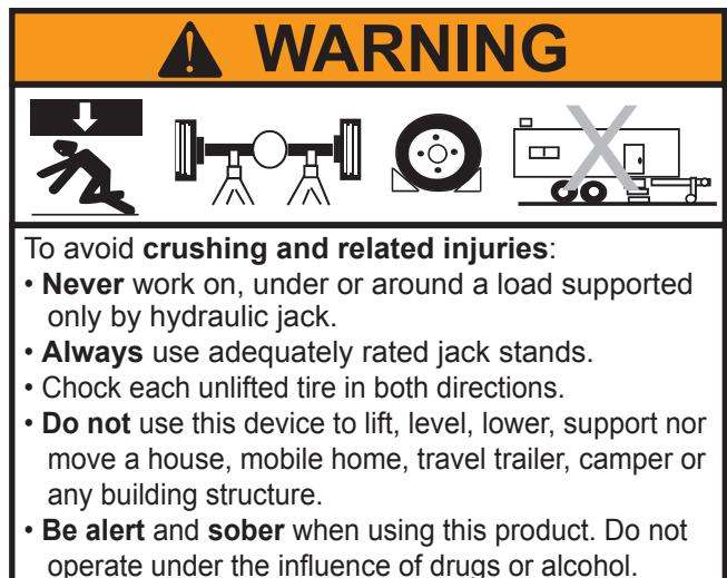
**!** Be sure all tools and personnel are clear before lowering load. Only attachments and/or adapters supplied by the manufacturer shall be used. Lift only on areas of the vehicle as specified by the vehicle manufacturer.
