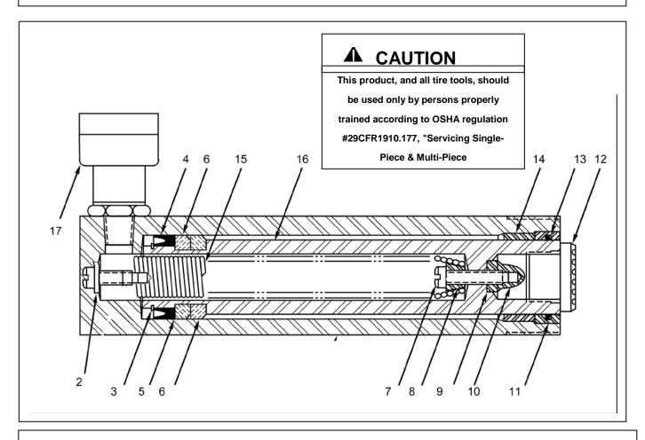
Note: Rod bearings (Item 6) to be assembled with splits staggered 90° apart.
