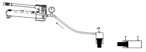
Single-acting cylinders: Position the cylinder so that the plunger is pointed down and the cylinder lower than the pump. Fully extend and retract the cylinder 2 or 3 times. Double-acting cylinders: Lay the cylinder on its side and have the couplers facing up. Fully extend and retract the cylinder 2 or 3 times.
