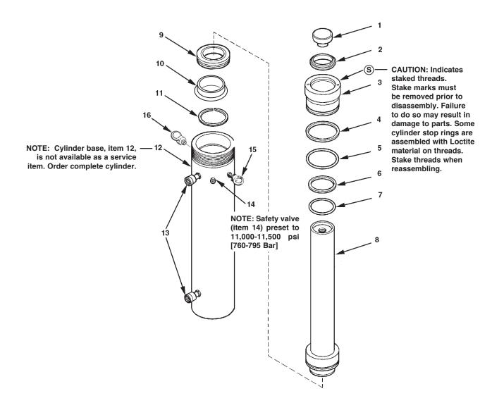
Figure 1, 100-ton, Double Acting, Solid Plunger Hydraulic Cylinders
