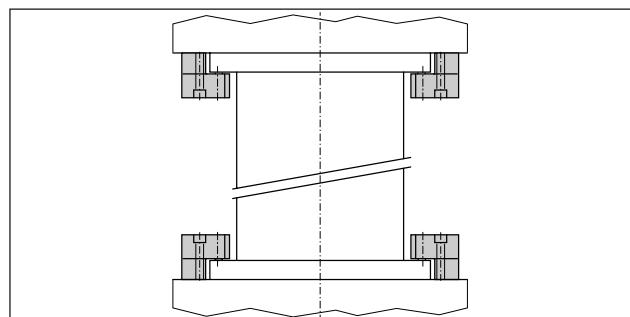
MLC-604, MLC-906 and MLC-1208 Modular Piston Manifolds are single-action spring return cylinders. They have been designed to clamp dies onto press forming tables. Depending on the model, these cylinders have a capacity of 60-90, or 120 kN. The dimensions are provided in illustration 2 page 13. The oilconnections are 1/4" BSP.
