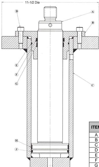
25 ton Workhead 4-1/2" Dia. Bore 3" Dia. Rod 10-1/4" Actual Stroke 10" Rated Stroke Total Wt. = 127#
