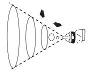
Spray pattern may be infinitely adjusted from round to flat.
