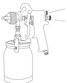
Spray width adjustment screw Turn right for round, left for fan.
