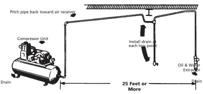
Oil and Water Extractor should be at least 25 ft. from the compressor, farther if possible.
