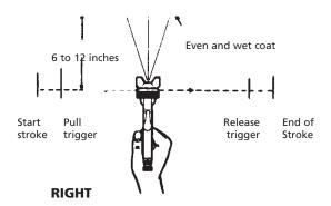
Hold the gun from 6 to 12 inches away from the surface depending on material and atomizing pressure. For a uniform finish, lap each stroke over the preceding stroke, making sure the spray is smooth and wet.
