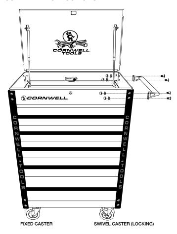
Mount push handle (Part #5) to the same side of the cart as the locking casters using the four stove bolts, washers, and nuts provided.
