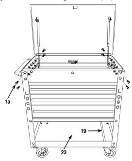
Step 14: Using 13mm socket completely tighten all fasteners!! Step 15: Insert spray can holder divider (#19) into provided cut away on the bottom shelf (#23). (Optional)
