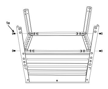
Step 7: Insert bottom shelf (#23) between the four legs flat side facing up towards the ceiling. Insert sixteen stove bolts (#1a) and completely tighten.
