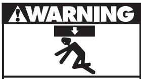
DO NOT OVERLOAD. OVERLOADING IS INDICATED BY BOWING EXTENSION TUBES OR SLIPPING ATTACHMENTS AND CAN RESULT IN PERSONAL INJURY OR DAMAGE TO THE EQUIPMENT.
