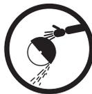
Always use the recommended wheel guard to prevent injury from broken grinding wheel parts. If a guard has withstood a wheel breakage, discontinue its use and replace it with a new guard. It may be damaged. Position the guard between the grinding wheel and the operator. Use barriers to protect others from wheel fragments and grinding sparks.
