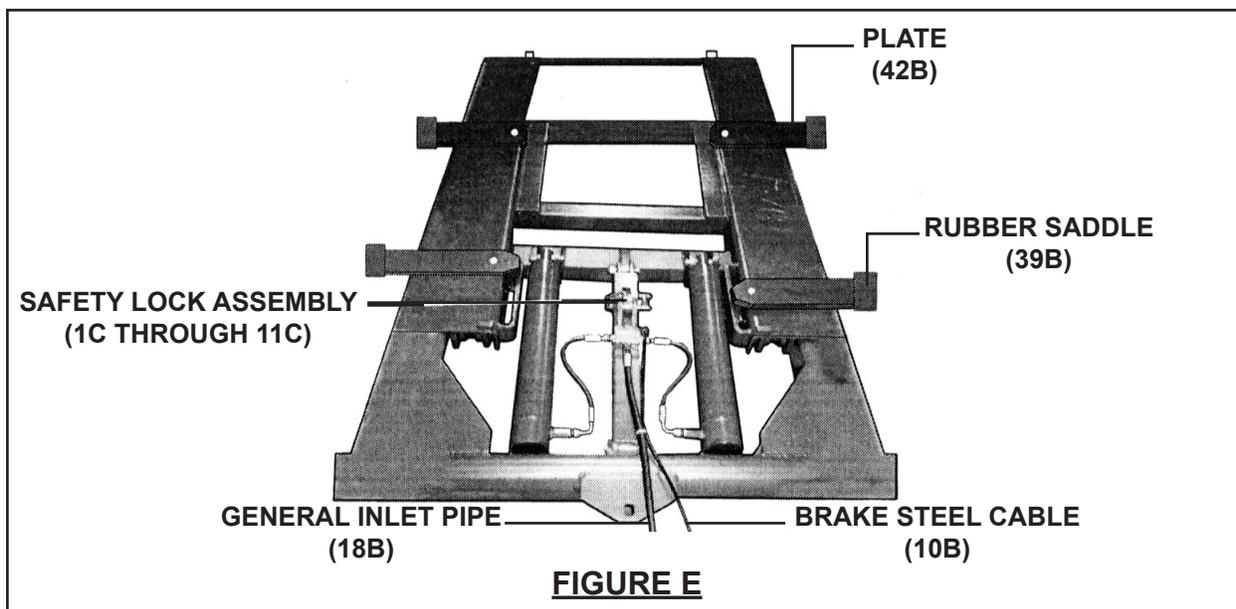
1. **⚠WARNING!** Never operate the Scissor Lift if the Safety Lock Assembly (1C through 11C) is not working properly. (See Figure E.)
