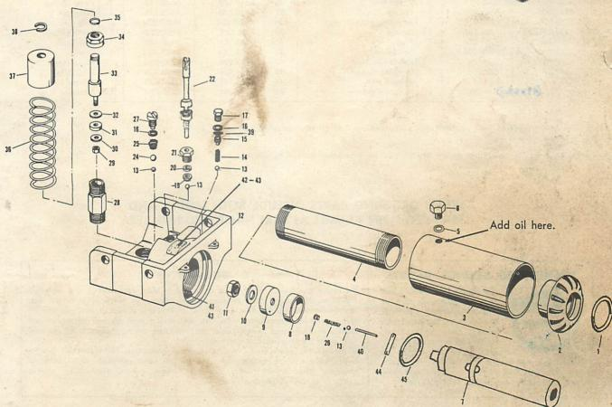
To Add Oil — Fully collapse ram plunger into power unit. Remove oil filling plug (item 6). Add LX-21 jack oil until about ¼ below top. Replace plug. If oil is dirty, thick, or gummy, remove and clean reservoir. Do not overfill as too much oil will cause faulty lifting due to lack of air space.
