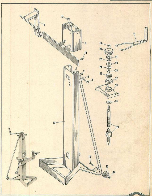
REPAIR PARTS SHEET FOR SJ-11
