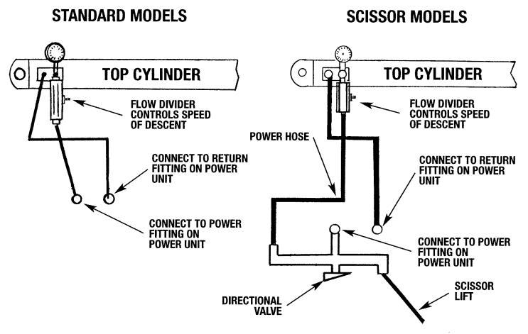
**FOUR POST MODELS WITH BUILT-IN SCISSORS** - The hydraulic hose that connects both scissor assemblies together, is stored underneath the ADJUSTABLE RAMP during shipment. Unwind hose. Route hose through the cutout in the side of the ADJUSTABLE RAMP. Connect to the hose protruding out of the STATIONARY RAMP using the double male fitting supplied. Teflon tape is recommended.
