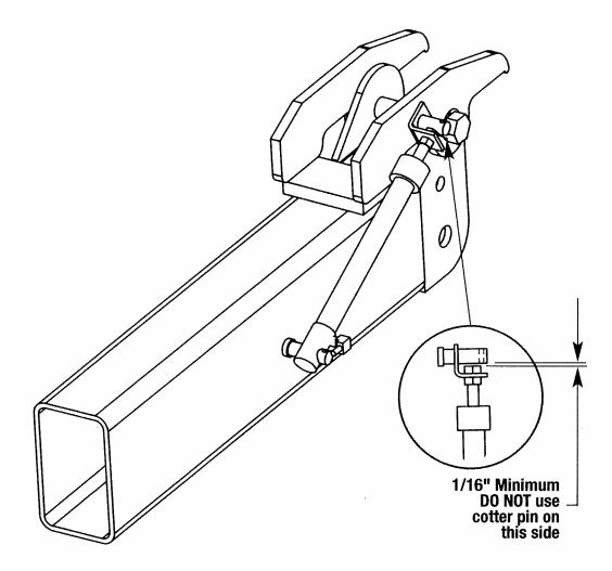
Before lowering the lift, each PRIMARY SAFETY must be raised to its fullest extent which will enable the safeties to clear the lattice descent. Once the lift reaches the floor all of the safeties will automatically reset.
