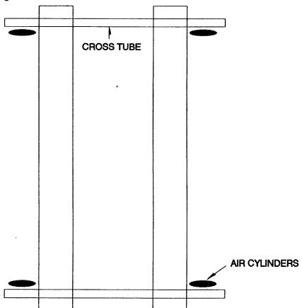
**NOTE:** It is helpful to rest the CROSS TUBES on the bottom lattices in the post prior to connecting chains.
