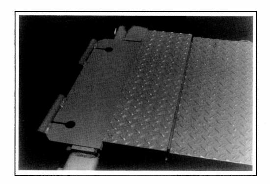
Place STATIONARY RAMP in position between locating blocks welded to the CROSS TUBES and adjacent to POWER BEAM. Place ADJUSTABLE RAMP in position on CROSS TUBES.
