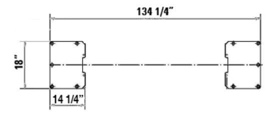
8. Use the existing holes in column base plate as a guide for drilling the 3/4" diameter holes into the concrete. Drill the anchor holes only for ONE column, installing anchors as you go. You will install anchors in second column after the cables, hoses, and cross beam are installed.
