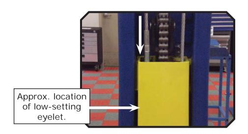
This is the Non-Powered side carriage. The arrow is where the cable from the Power side comes down. For the Highest setting, use the eyelet at the top, left hand corner. For the low setting, directly below the top eyelet, there is a second eyelet inside the carriage. Pass the cable through the top eyelet and bolt into the inner, hidden eyelet. Just be sure cables do not cross and do not tighten the cable nuts down until they are run around the pulleys.
