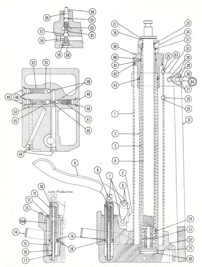
**NOTE** - When new base is required, order P/N 225380 and add P/N 225382 pump cylinder. Early production base and pump cylinder were one piece. Late production has removable pump cylinder.
