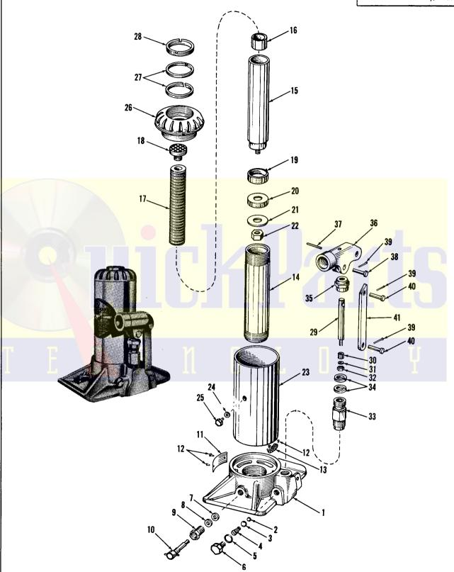
REPAIR PARTS SHEET FOR CB-9D HYDRAULIC JACK
