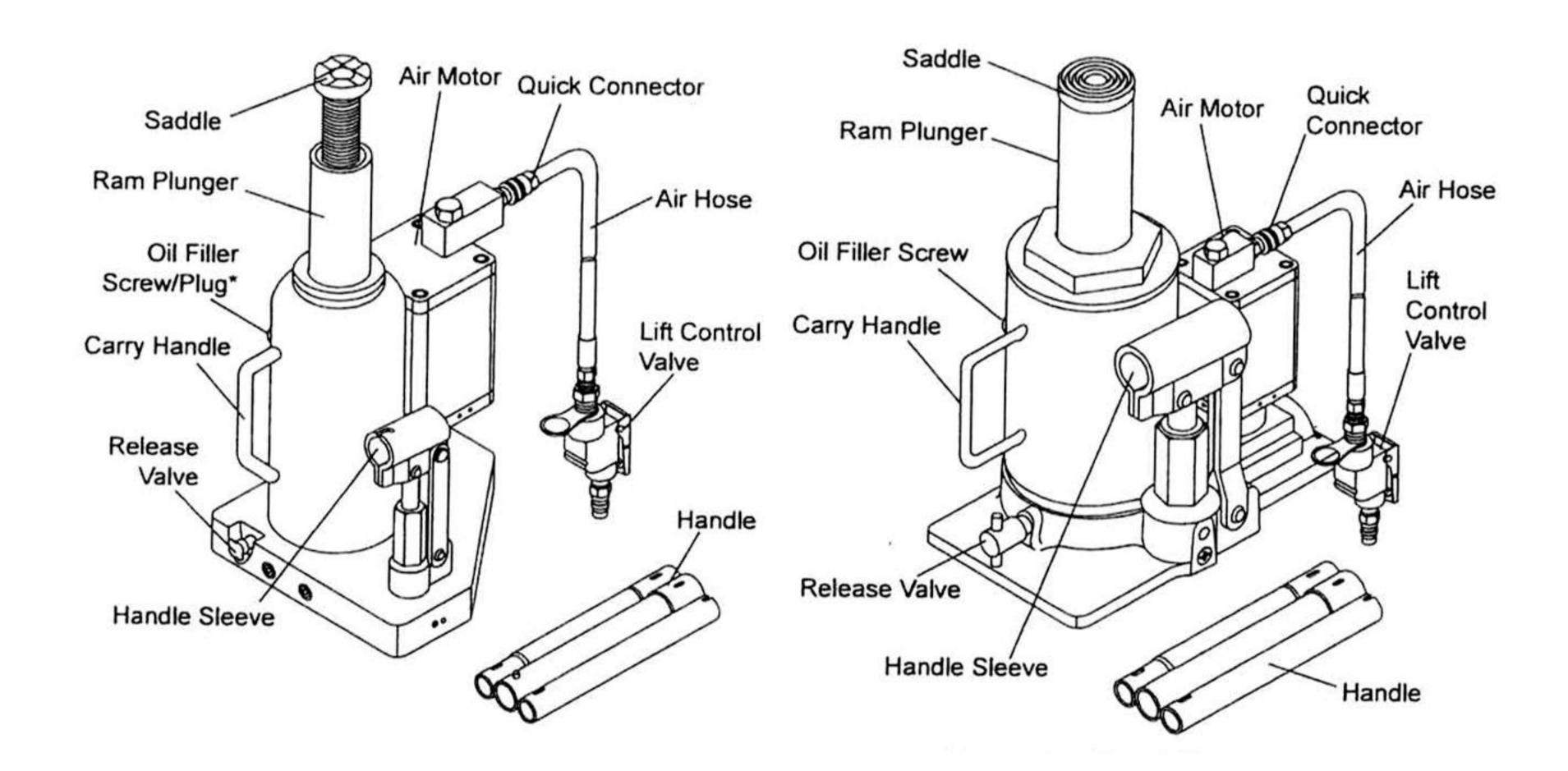
If the air motor runs but the jack won't lift try bleeding air out of the jack according to these instructions.
